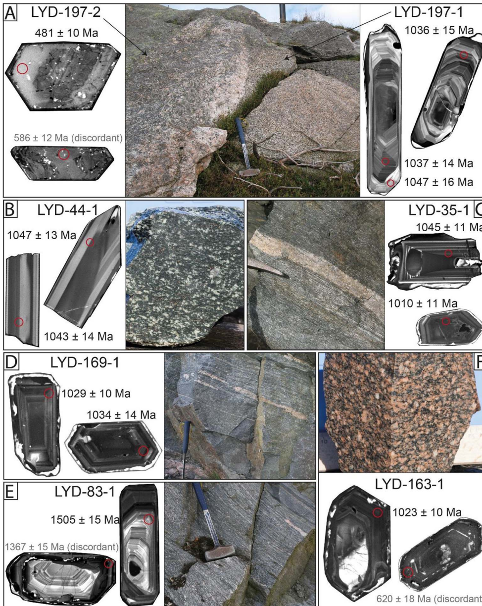
Fig. 7. Geochronology sample lithologies and representative CL images of analyzed zircon grains. Note the distinct textures of zircons from granitic (A, D, E), gabbroic (B, C) as well as highly radioactive leucogranitic samples (A, F), respectively. Analyzed spots (15 \mu\text{m} diameter) are shown by red circles together with resulting single grain Concordia ages. Note that discordant ages (grey) are not geologically significant. (For interpretation of the references to colour in this figure legend, the reader is referred to the web version of this article.)
